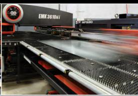
**EMK 3610 NT** — Servo-electric turret punch press that enhances productivity by providing additional functions such as contouring, deburring, slotting, marking and forming.
