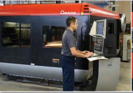
LC 3015 FINT — Featuring a 3-axis linear drive system, no lens change technology plus ultra-fast piercing and cutting, the LC-FI NT provides exceptional productivity.
